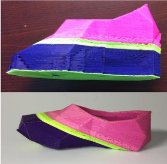
**Figure 1:** Printed shoe with support material and support material removed.
